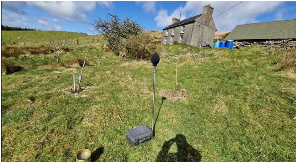
Plate 12-2 Noise monitor Installed at NML2
