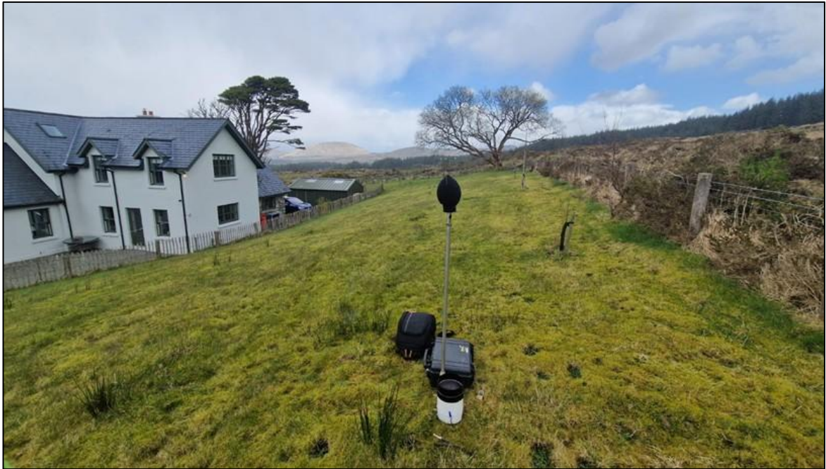
Plate 12-5 Noise monitor Installed at NML5
